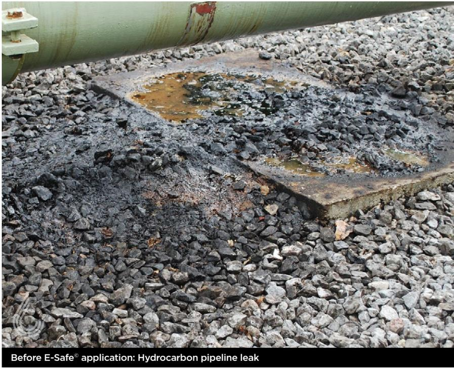
Before E-Safe® application: Hydrocarbon pipeline leak
